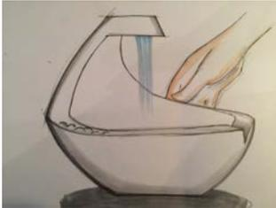
Figure 2. Illustration of concept sink. The sink is controlled by gestures along the edge of the basin. The materials of the sink are designed to ware demonstrating traces of use.
